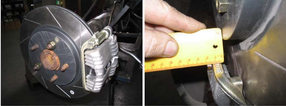
Caliper protrudes 17mm past hub face; check that your wheel has sufficient centre/spoke clearance.
