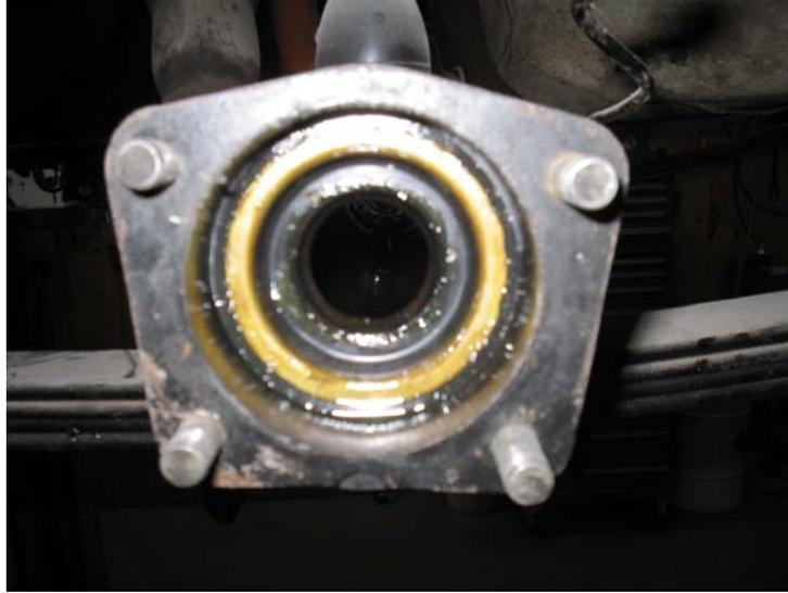
Holden end flange pattern is shown, note this unit has special bored out housing for Ford ball bearings and internal seal, Holden use Taper Roller Bearings and external seal! Differential specialists often mix and match flanges when making conversions so you need to check how they did your conversion, what end pattern and what bearings they used as anything is possible.
