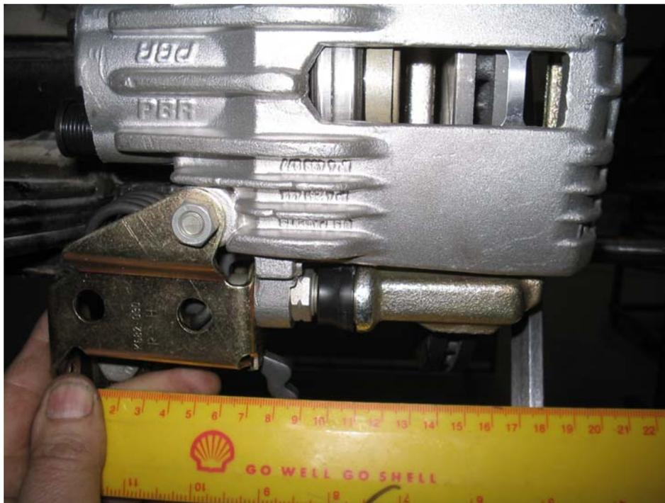
174mm required from end of bare axle to caliper handbrake bracket
