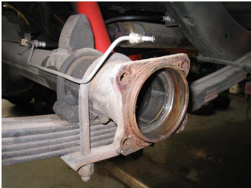
2/ Big Bearing 9 inch, 2.375" by 3.5" bolt pattern with 3.150" bearing diameter.
