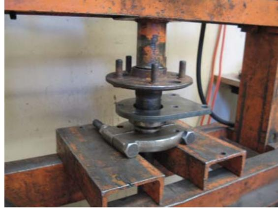
Bearing being pressed on, new plate in place.
