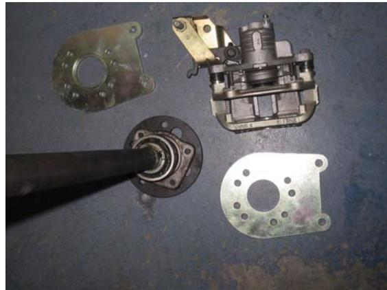
The disc rotor used on this application is a 300mm by 28 thick item originally intended for late model Ford Mustangs, bought off DBA as blanks so we can match your existing stud pattern. This rotor has a late Ford centre hole spigot, should you have an early small centre axle we supply special shouldered wheels studs which locate the rotor on the studs. Calipers come in left and right and so can be forward or rear mounted or even a pair of LH units supplied for staggered shock applications.
