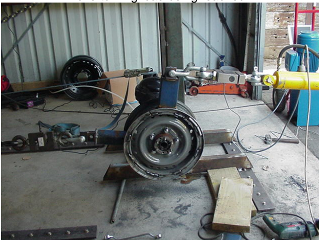
Test rig simulating 2g vertical load and 1.2g braking load. Note that disc calliper and rotor assembly was pinned through the centre of the calliper piston to prevent rotation of the hub and brake disc assembly. This test also tests the strength of the calliper mounting bracket.
