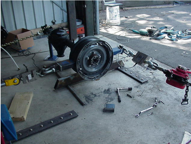
Test rig simulating 1g vertical, load and -0.6g lateral rut load
