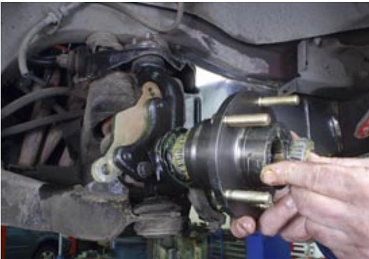
**STEP 07** Before installing the Hoppers CNC-machined hub, thoroughly grease the inner and outer bearings. Put the larger inner bearing on the spindle, then, after packing the inside of the hub with grease, set it into place. Next push the small bearing firmly into the outer cone of the hub, then the retaining washer and finally the castellated nut. The photograph summarises the basic order of the steps.
