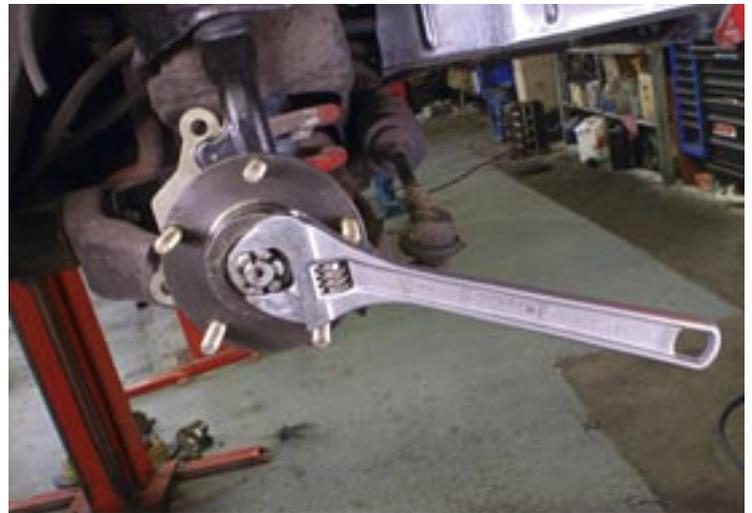
**STEP 08** How tight should the bearings be? The hub must turn freely but shouldn't wobble or rock — the only movement must be rotational. Very gently nip up then back off the nut a couple of times, while turning the hub. For final tightening, use nothing more than the weight of a big shifter. Flip the nut-retaining cage around until the holes line up and make sure you use a new split-pin to fasten it.
