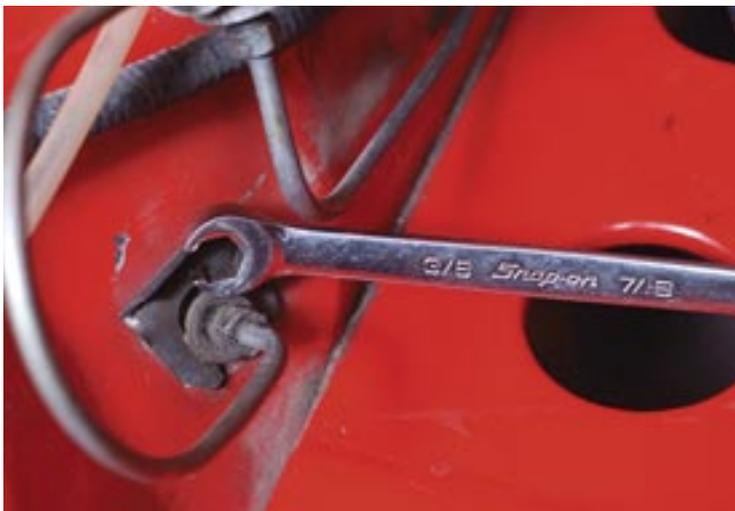
**STEP 11** Standard rubber hoses (that run up to the inner guard) have been upgraded to stainless. Whenever loosening or tightening brake lines and fittings, always use a proper flare-nut spanner. Using an open-ender commonly results in damaged fittings, especially if they've suffered past abuse. It's probably also a good idea to fit a new master cylinder, though we haven't included it in this issue.
