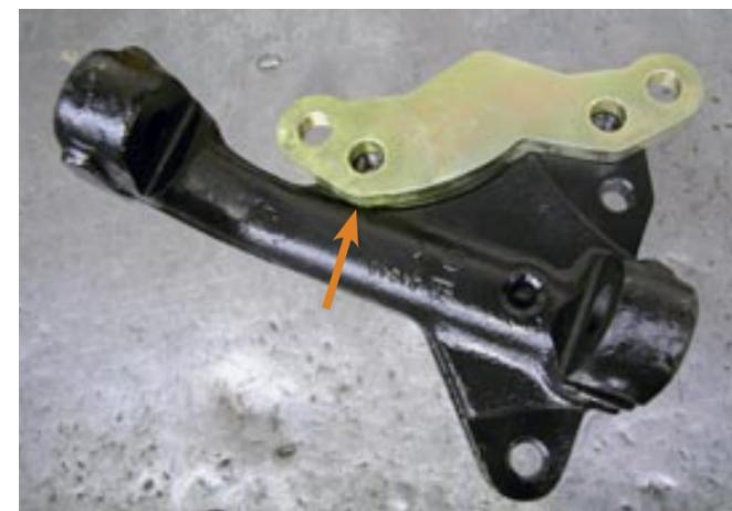
**STEP 04** Before installing the stubs (or while you're swapping them from left to right), check the adaptor plate holes line up with the stub-axes. Sometimes insufficient material has been machined from the area indicated by the arrow. If necessary, grind back some metal in this raised area so they fit — remove just enough so the holes line up but do not grind the machined area.
