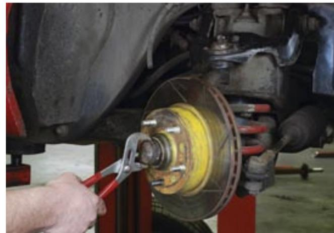
**STEP 01** The first step is to remove the existing brake system, whatever it may be. Jack the car up, remove the wheel and clamp the brake line. You can get cheap brake-hose clamps from any auto-parts outlet. Now disconnect the line from the caliper, remove the caliper, remove the dust cup, safety split-pin securing the spindle nut, the spindle nut itself, the disc, bearings and so on.
