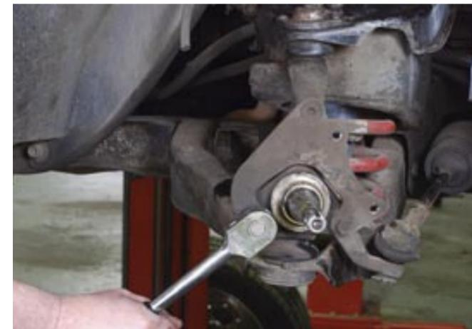
**STEP 02** Undo the two bolts connecting the steering arm to the stub-axle. This car had been fitted with Torana drum-brake spindles and an adaptor to accept HQ brakes — the adaptor plate is visible in the shot. These stub-axles had to be removed and replaced with standard LH-LX Torana disc-brake stub-axes, as the Hoppers Stoppers kit doesn't fit the drum-brake stubs.
