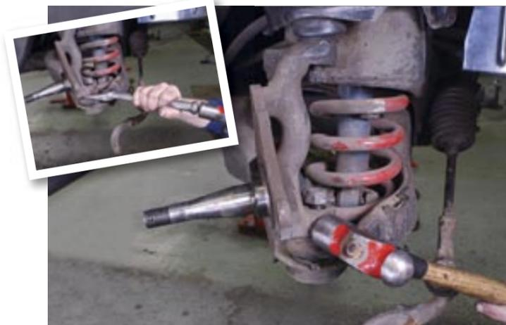
**STEP 03** Ordinarily, the stub-axes are removed and swapped side for side so that the calipers become rear-mounted instead of front-mounted. Partially undo the ball-joint nut, so about half of the thread remains engaged, and give the side of the stub axle a couple of firm whacks with the hammer. If the ball-joints do not dislodge, use a ball-joint (tie-rod) breaker fork, as shown in the inset.
