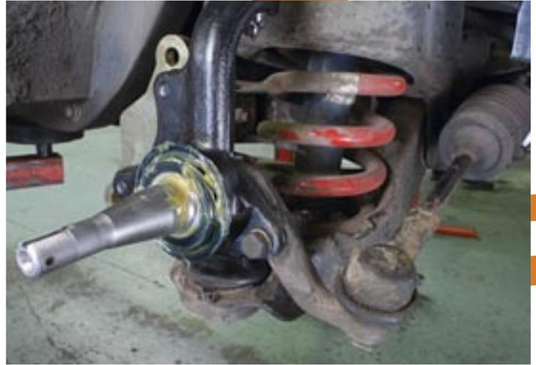
**STEP 06** Once the stub is refitted and the ball-joint tightened, the stand can be removed. Refit the steering arm. The seal for the inside of the replacement hub isn't placed into the hub as in other kits. Rather, it fits onto the inner end of the spindle as shown here. Make sure the spindles are scrupulously clean before fitting anything to them as even the smallest debris will quickly kill the bearings.
