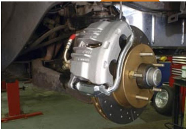
**STEP 12** Make sure the anti-rattle shims are fitted and centred in the caliper brackets (note them in Step 9) and make sure the hub face is clean before slipping on the rotor. Then bolt the caliper in place and hook up the brake hose. The calipers in the kit are marked left and right. Ignore this and ensure the bleed nipples are on top of the calipers. This is absolutely essential.
