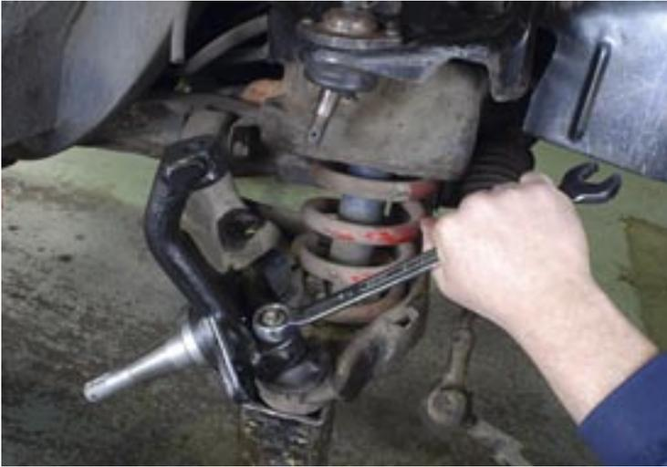
**STEP 05** This is the replacement stub going in. Make sure the ball-joints are tight as they can actually snap off if allowed to move about on the taper. Note that a stand has been placed under the lower control arm to keep the spring compressed. Doing this allows you to remove the stub-axle without having to remove the spring. You could use an axle-stand to do this.
