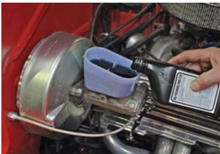
**STEP 14** This is a good time to renew all the fluid (which you should do every couple of years anyway). After topping up with fresh fluid, Peter prefers to gravity-bleed the system; open the master cylinder, crack the top bleed-nipple and wait. The fluid pushes air up and out through the top of the caliper. When fluid emerges, seal the system and it's likely you'll have a firm pedal.
