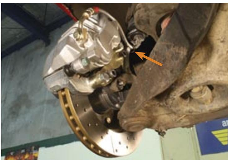
**STEP 13** The brake hose has to be secured at the top of the stub-axle with a cable tie (arrow). When everything is fitted, turn the wheels from lock to lock and check clearances. Do the same with the car on the ground. The pads should also be checked to make sure they don't hang off the outer edges of the rotors. Note the new split-pins in the ball-joints — never re-use any split-pin.
