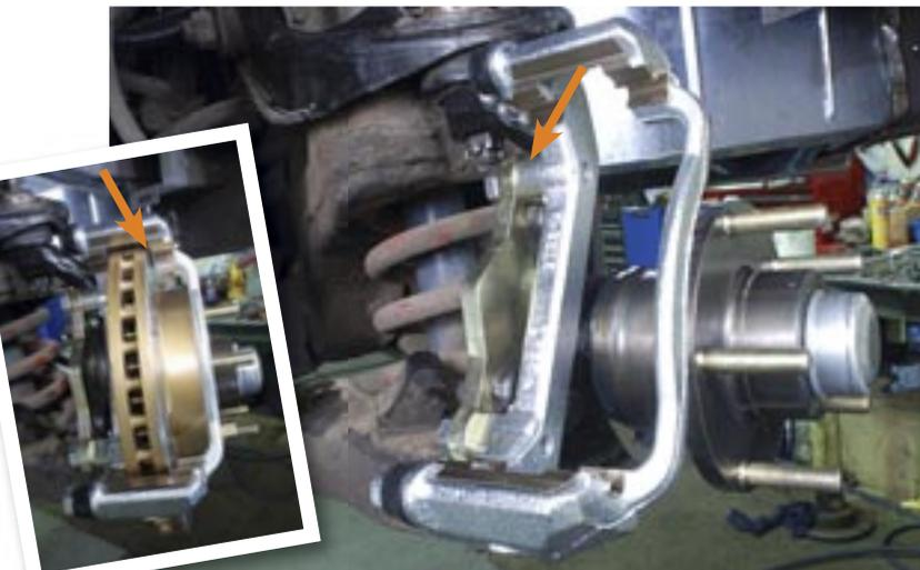
**STEP 09** Bolt up the caliper bracket using the supplied spacers (arrow) and slip on the rotor. Nip up a couple of wheel nuts to snug the rotor into position so you can check if it runs in the middle of the bracket (inset arrow). If the disc is too far outboard, remove the spacers and add the supplied shims between them and the bracket until the disc runs centrally within the bracket.
